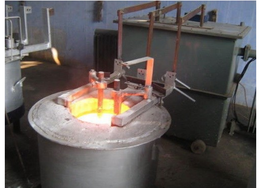
Fig. Salt Bath Furnace
