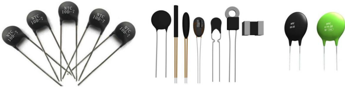
Fig: Different types of Thermistors and Construction
