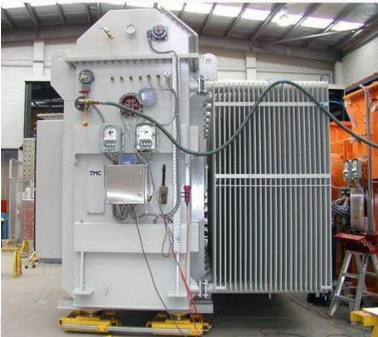
Fig (c): Oil Natural Cooled Rectifier Transformer
